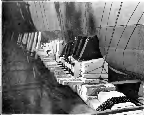
Fore poppet of the President Hoover showing the plate saddles and methods of shoring employed.
